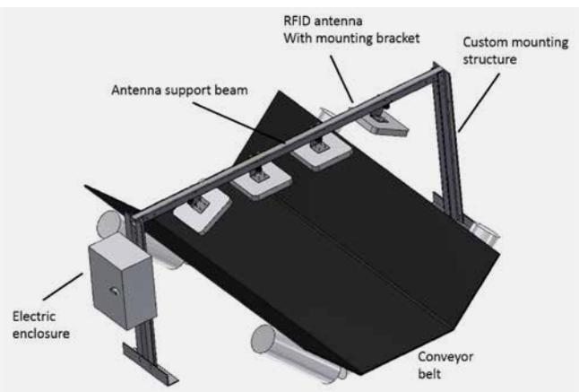
**These images show the antenna array at the exit from the screen house. The antennas detect if a screen media panels becomes dislodged.**
